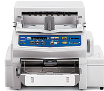
Bell & Howell 8140DCI Spectrum XF Scanner, an example of a (circa 2008) Commercial off-the-shelf (COTS) high-duty cycle scanner capable of 140 pages per minute, scanning both sides of the page at 200dpi resolution. It has a 500-sheet input capacity.
