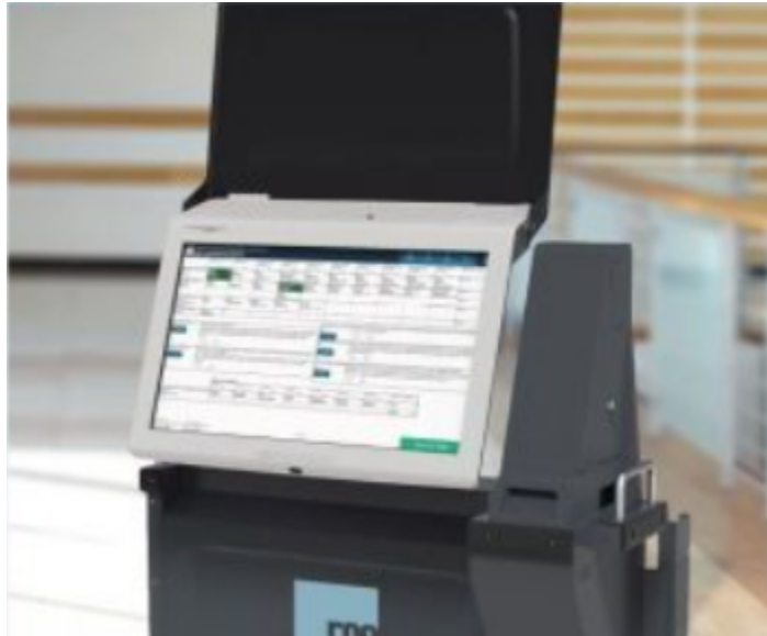
Figure 5. ES&S ExpressVote XL BMD with attached ballot summary card printer (and reader).
