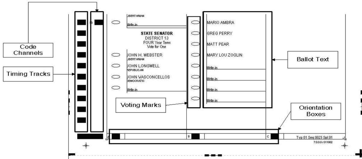
Figure 2-2: Machine-Readable Components on ESSIM Ballot
