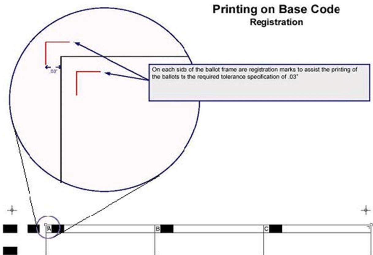
2. Turn the ballot over and do the tests again on the back of the ballot. If all three tests on each side fall within tolerances, the scanner will be able to read the ballot.
