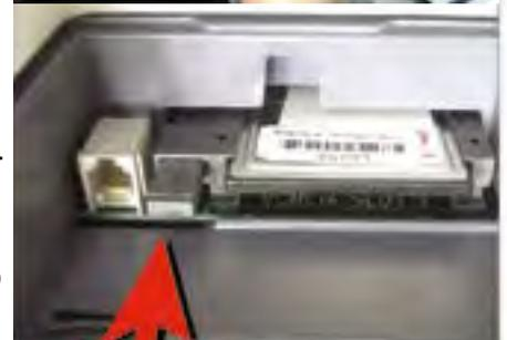
6. Press the black rectangular button to release the memory card, then SLIDE the memory card out.
