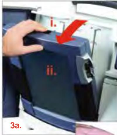
**3a.** With your left hand, press down on black button (i) on top of the tablet (ii), and lean the tablet towards you. **DO NOT LIFT THE TABLET OUT OF ITS CRADLE.**
