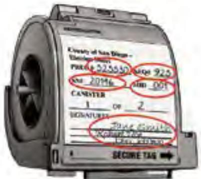
7. The canister should be, and remain, sealed with a blue security seal. Ensure that the canister label is filled out completely
