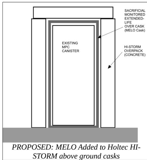
Above-ground systems can add the MELO Cask fairly easily by removing the outer concrete overpack and adding the MELO Cask, and then adding a new, larger concrete overpack.
