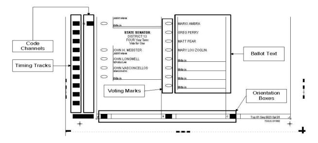
Figure 2-2: Machine-Readable Components on ESSIM Ballot
