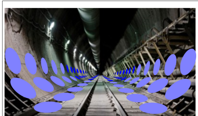
YM-HELM Concept – Radial HELM storage in the YM main tunnel so each cask can be monitored, serviced and replaced, to accommodate 120,000 tons heavy metal waste (roughly 10,000 casks). Each blue circle represents the lid of a below-grade cavity where the cask is interred.
